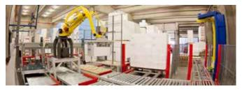
because June is a busy month). The end piece, the stacking robot, was put in standstill in August 2011 and successfully started up. The gain in speed on the packaging line is big, with this line one can manage 60 m<sup>3</sup>/hr and for some types up to 80 m<sup>3</sup>/hr, thus twice as much as earlier. The night shift can thus be dispensed with.
